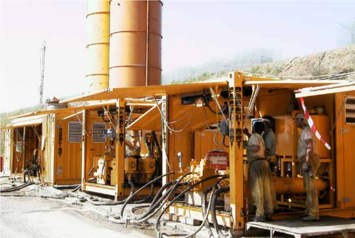
Fig. 10. Pacchiosi mixing and injection installations.
