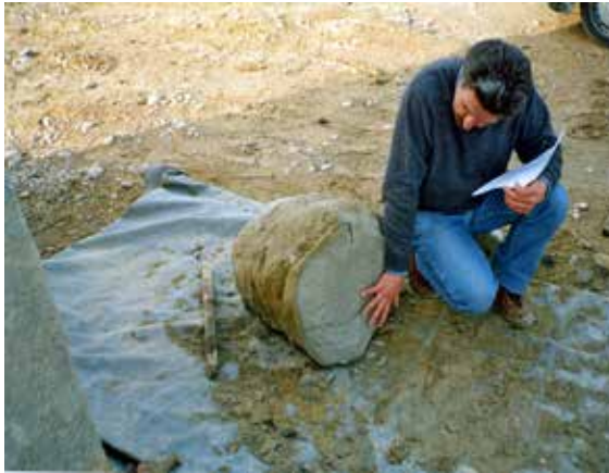
Fig. 3. View of Jet Grouting column from test field.
