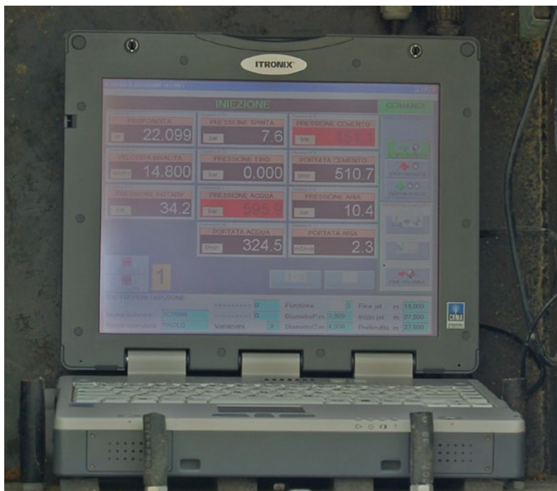
Fig. 27. Computer installed on the perforating machine; view on the monitor of characteristic parameters.
