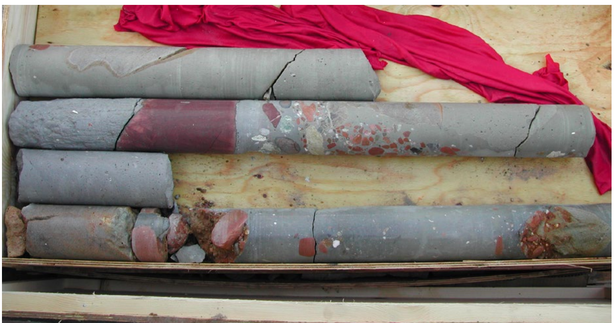
Fig. 22. Example of core sampling; note the perfectly cemented inclusions
