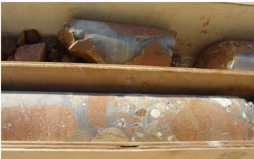
Fig. 20. Example of core sampling; note the perfectly cemented inclusions
