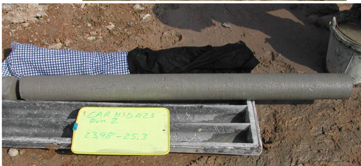
Fig. 25. Example of core sampling; note the perfect uniformity and continuity of the treatments performed
